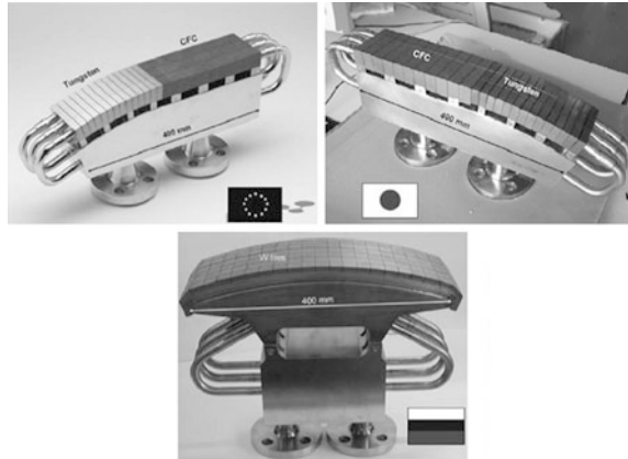
Fig. 4.27 ITER vertical target ( top ) and dome ( bottom ) medium-scale prototypes. Reprinted from Ref. [3], Copyright 2010, with permission from Elsevier
