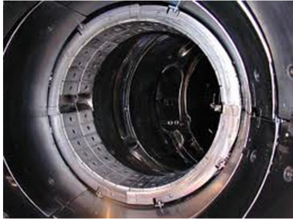
Fig. 4.23 HT-7 fully circular poloidal limiter
