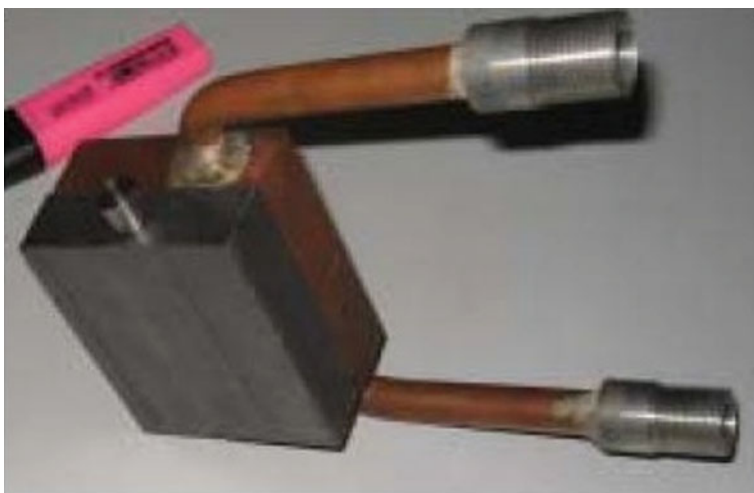
Fig. 4.36 Thermal test sample for EAST divertor
